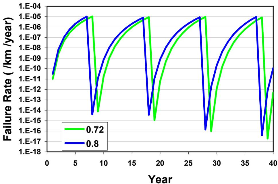
Figure 8. (48) Comparison of Failure Rates between 0.72 and 0.8 Design Factors (for corrosion defects): Effect of In Line Inspection.
