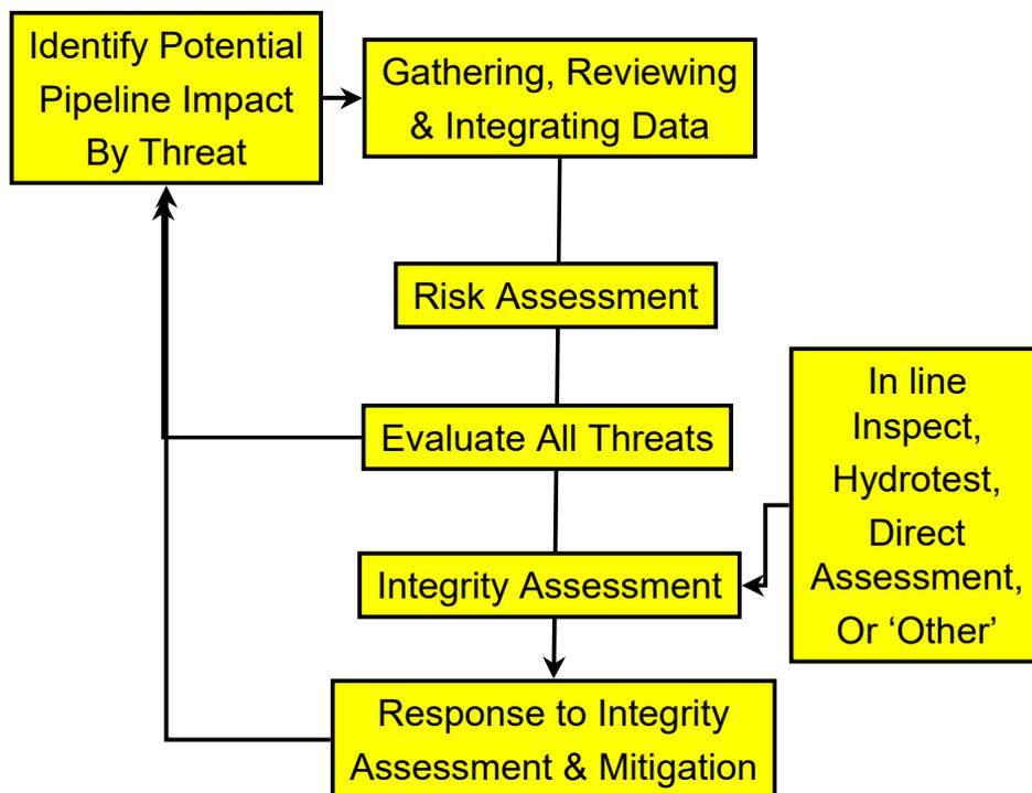
Figure 2 (12). Integrity Management Process Flow Diagram from ASME B31.8S.
