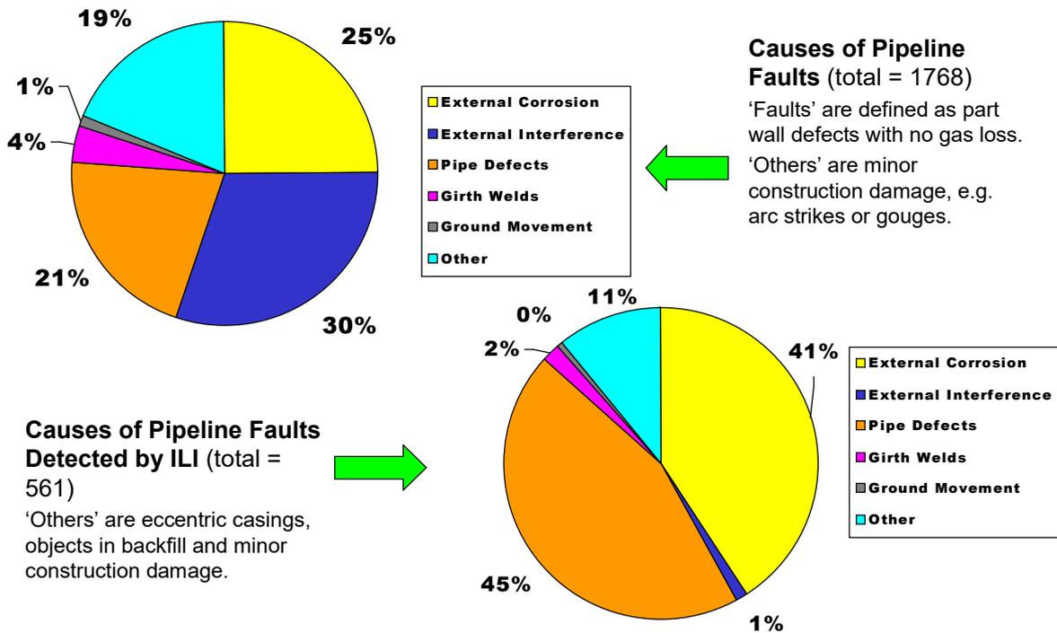
Figure 7 (14). In Line Inspection and the Defects it Detects.
