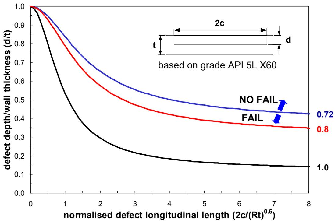
Figure 3. Theoretical Failure Relationship of a Part Wall Defect (under internal pressure loading).
