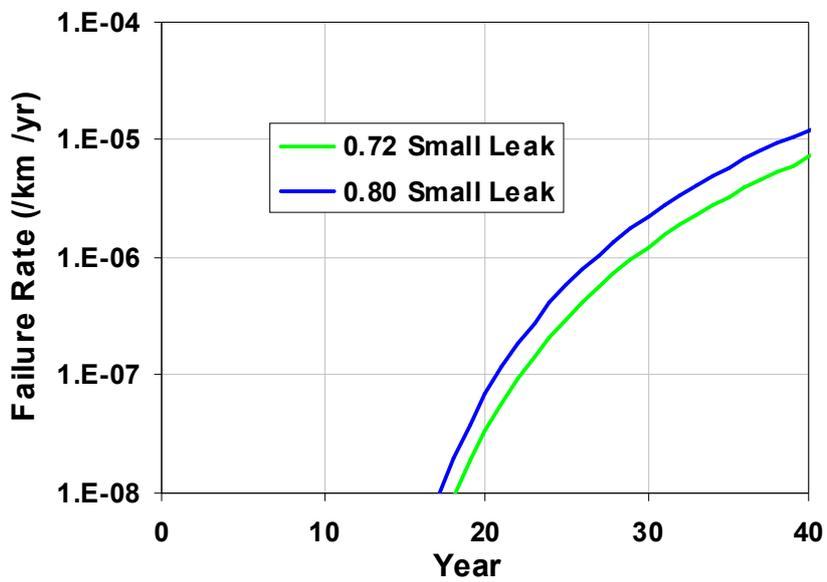
Figure 6 (48). Failure Rates for Corrosion Defects at Two Design Factors.
