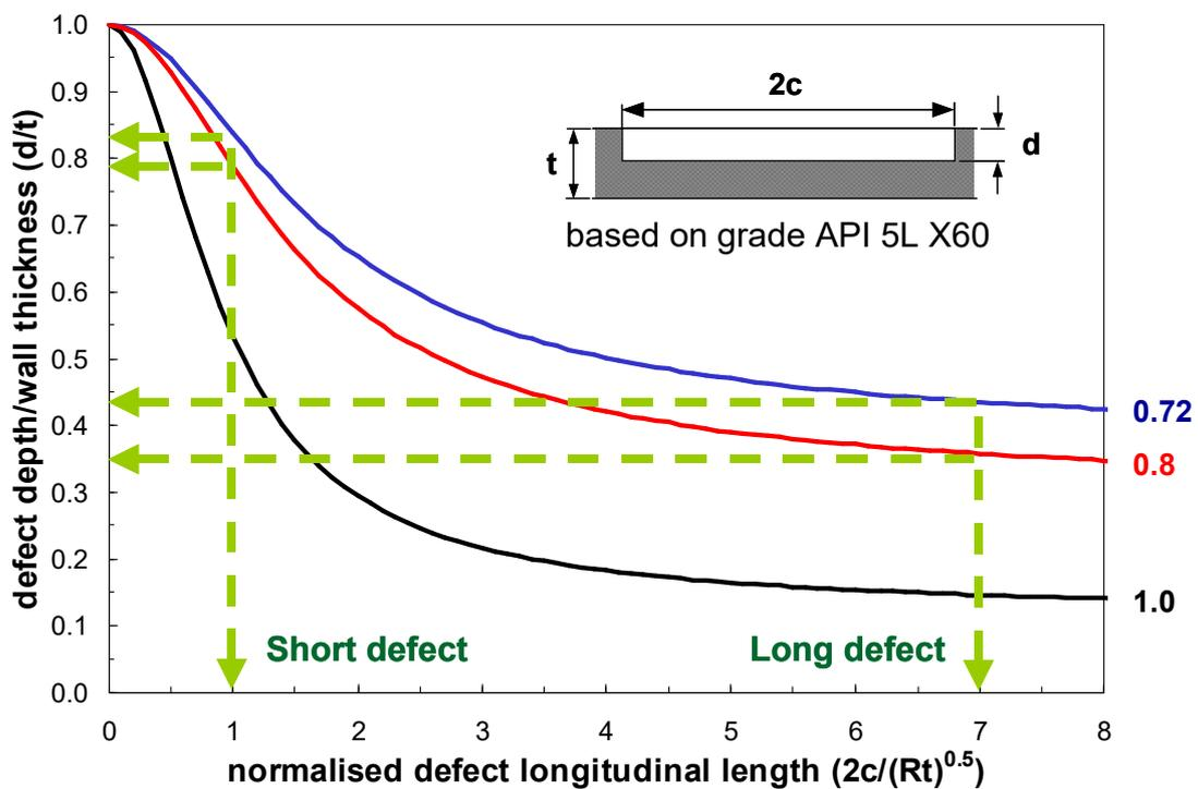
Figure 4. Effect of Increased Design Factor: Smaller Defects Fail at Higher Design Factors.
