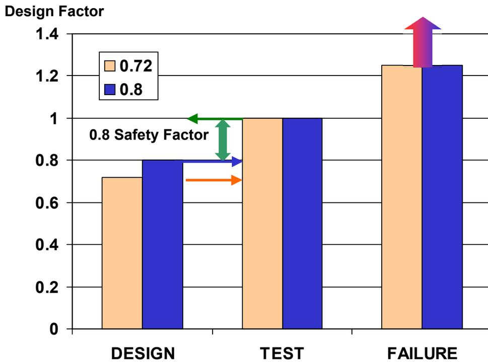
Figure 9. Reduction in Safety Factors with Increasing Design Factor.
