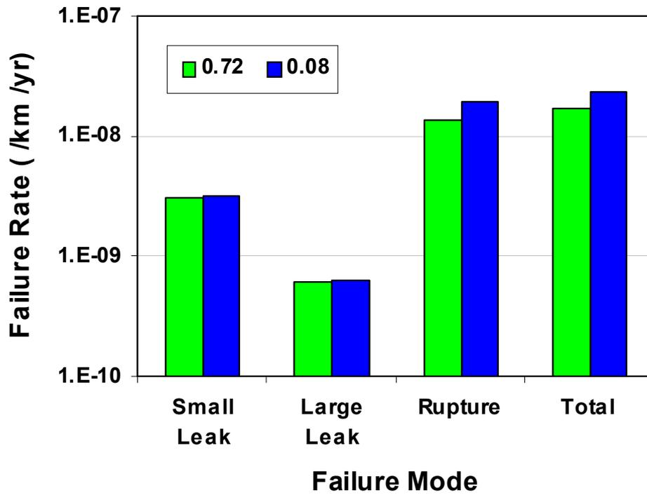
Figure 5 (48). Calculated Failure Rates for Mechanical Damage at Two Design Factors.
